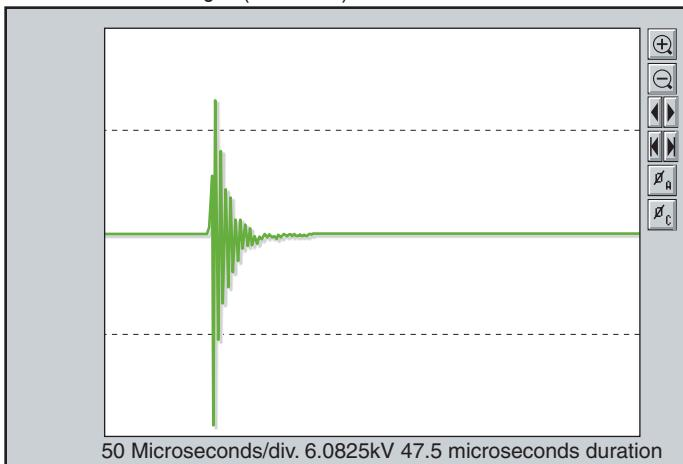
**Fig. 1.** A voltage transient is a high-rising, short-lived voltage on one or more phases of a system and can reach 20,000 volts or more. Although they can originate outside the facility, 80% come from inside the plant, with sources being photocopiers, arc welders, lighting and even the switching of a circuit breaker.
